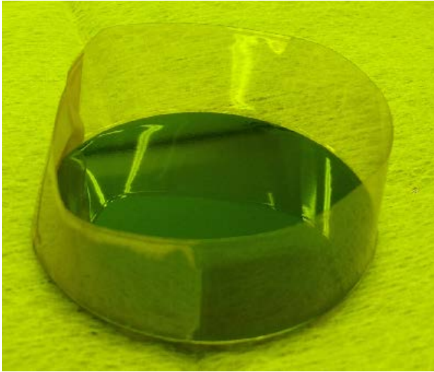
Fig. 4: Mold enclosed with peripheral wall of polyimide.
