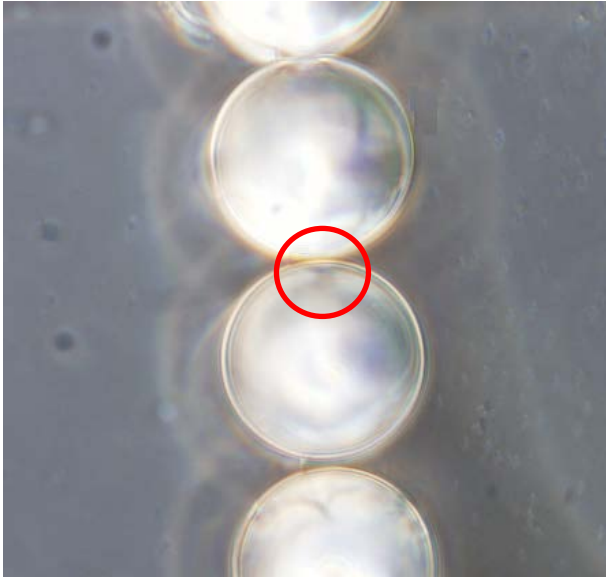
Fig. 18: Red blood cells flow through micro slits of type 2. The diameter of columns is 0.05 mm.
