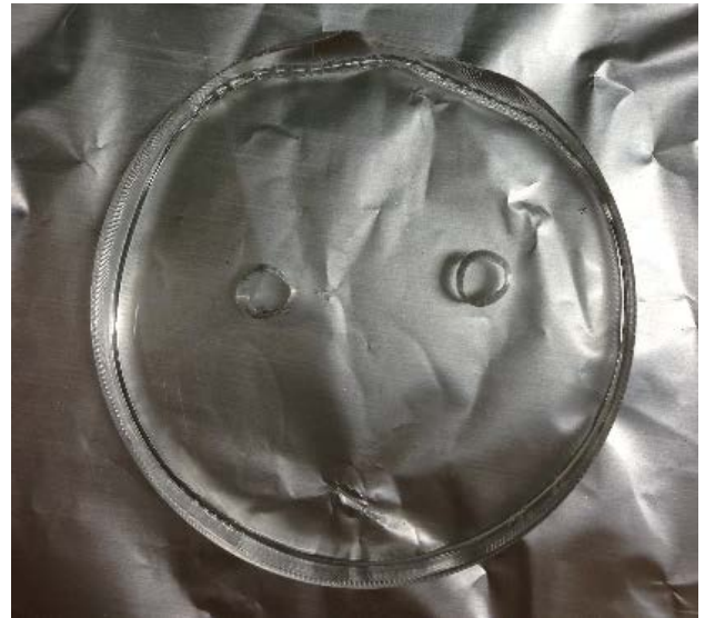
Fig. 8: Upper disk of PDMS with two holes for connection with tube.
