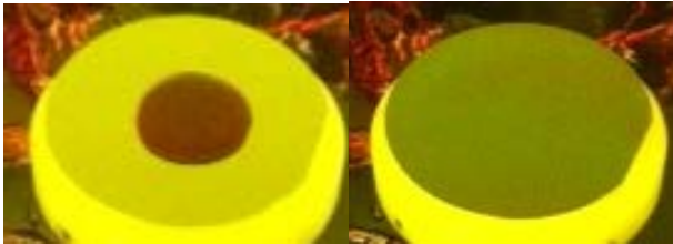
Fig. 2: Photo-resist material on wafer: before (left) and after spinning.
