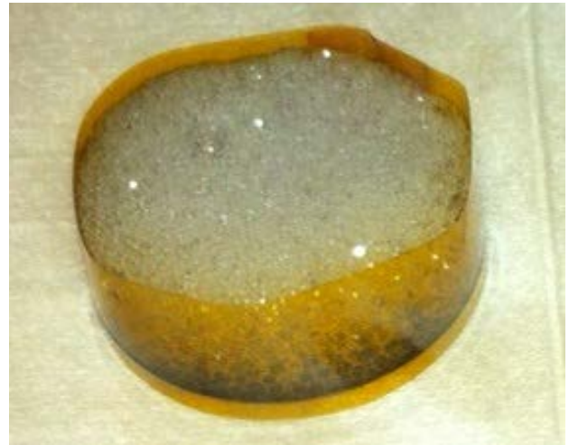
Fig. 3: Degassing of PDMS on mold of silicon wafer with micro pattern.
