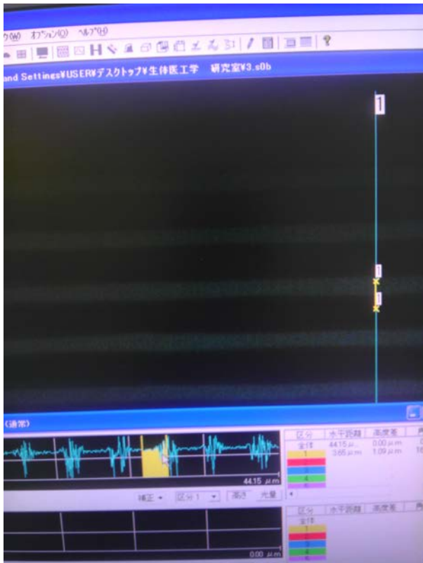
Fig. 9: Dimension of the micro groove (D) measured with a laser microscope.
