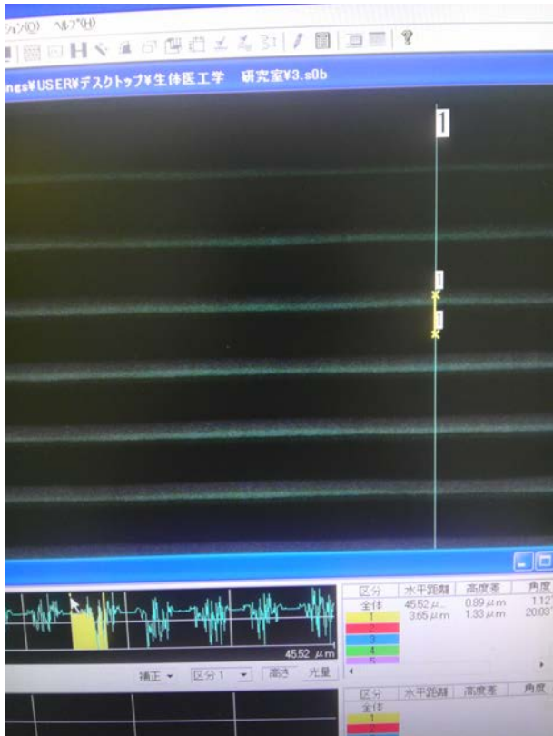
Fig. 8: Dimension of the micro groove (C) measured with a laser microscope.
