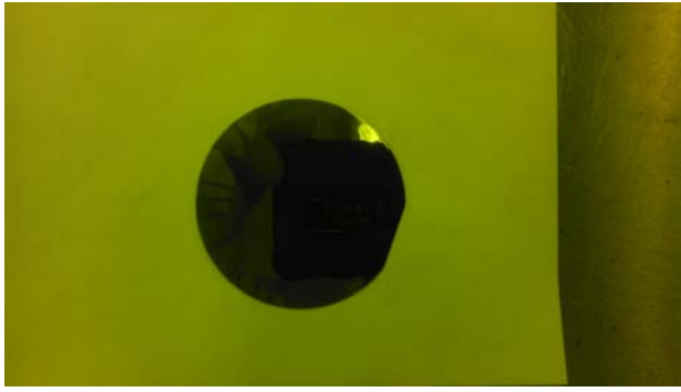
Fig. 2: Silicon wafer coated with photo-resist material.
