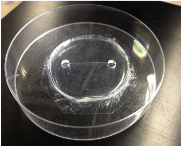
Fig. 5: The flow chamber consists of thin silicone rubber sheet sandwiched between transparent polydimethylsiloxane (PDMS) disk and culture dish.
