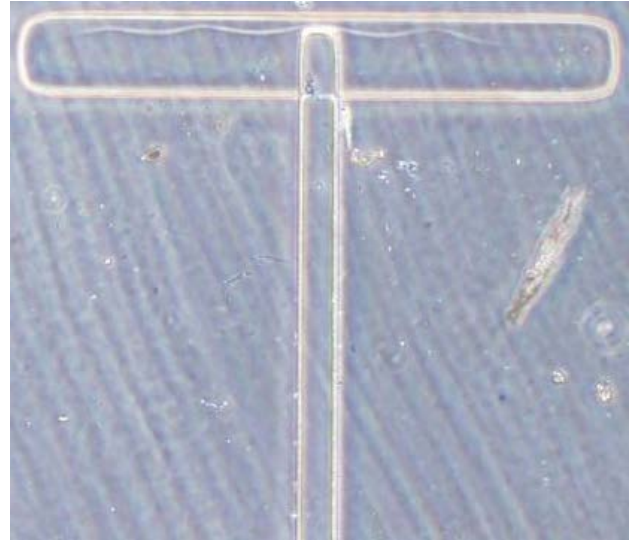
Fig. 5: Micro slit. Cells flow from left to right under vertical ridge (0.05 mm height). Horizontal ridge has 0.001 mm height (1 mm length, 0.1 mm width).
