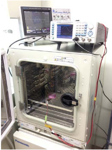
Fig. 6: Sinusoidal voltage is transmitted to the piezoelectric element from function generator placed outside of the incubator.
