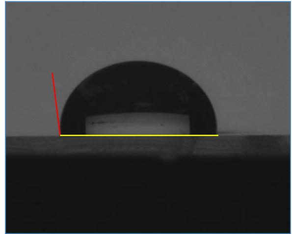
**Fig. 7:** Contact angle (1.7 rad) on the surface of PDMS before oxygen plasma ashing.
