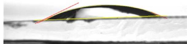
**Fig. 9:** Contact angle (0.45 rad) on the surface of PDMS after oxygen plasma ashing.
