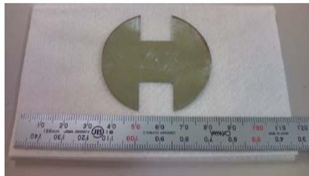
Fig. 1: Mask of aluminum for deposition.
