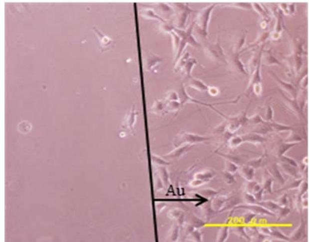
**Fig. 16:** More cells adhere in the gold film area (right half) on the surface of PDMS. Dimension from left to right is 1 mm.
