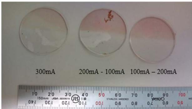
**Fig. 6:** Gold was deposited on the half of the surface of PDMS disk (upper half in the figure) by three kinds of sputtering process. 300 mA (left), 200 mA followed by 100 mA (middle), and 100 mA followed by 200 mA (right).
