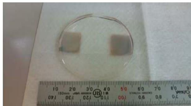
Fig. 2: Deposited gold film on the surface of PDMS.
