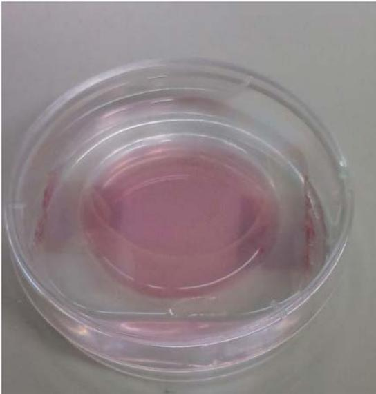
**Fig. 5:** Culture dish of PDMS placed in polystyrene dish of 70 mm diameter.
