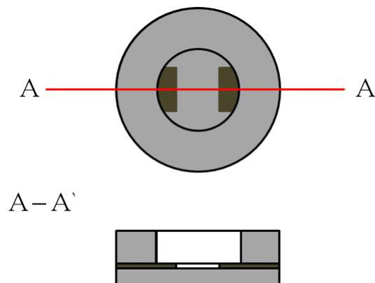
Fig. 3: Design of culture dish of PDMS. Cross-section at line of A-A' (bottom).
