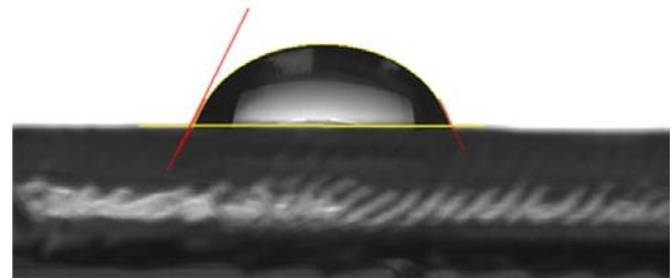
**Fig. 8:** Contact angle (1.1 rad) on the surface of gold sputtered (300mA) area on PDMS before oxygen plasma ashing.
