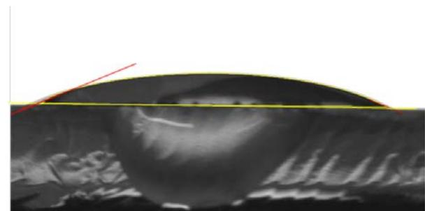
**Fig. 10:** Contact angle (0.38 rad) on the surface of gold sputtered area on PDMS after oxygen plasma ashing.
