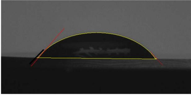
**Fig. 11:** Contact angle (0.80 rad) on the surface of gold sputtered (100mA & 200 mA) area on PDMS before oxygen plasma ashing.
