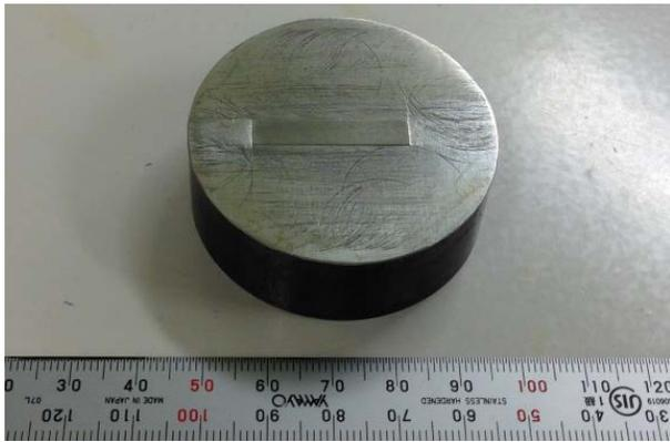
Fig. 2: Die of steel with a central rectangular convex.
