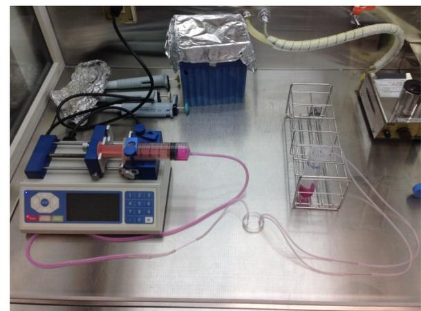
Fig. 5B: Medium is introduced into channel with syringe pump.
