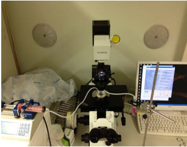
Fig. 4: Flow test system: pump (left), channel (middle), and microscope.
