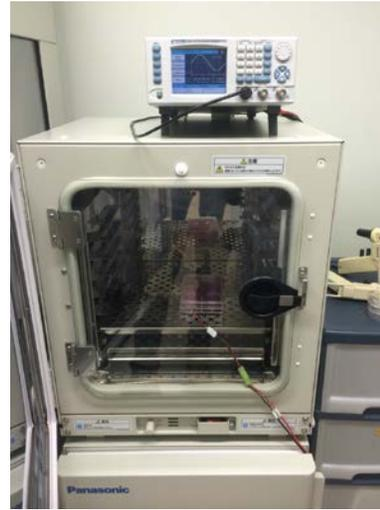
**Fig. 7:** Piezoelectric element in incubator is vibrated by function generator.
