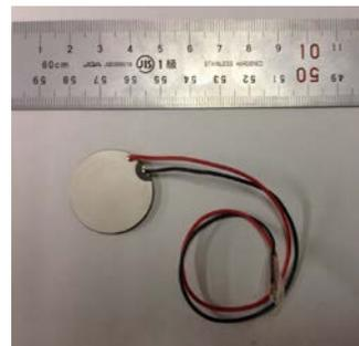
Fig. 1: Piezoelectric element.
