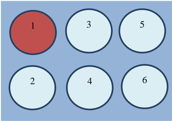
**Fig. 2:** Position of each well in the culture plate. Piezoelectric element is attached on the back of the well “number one”.
