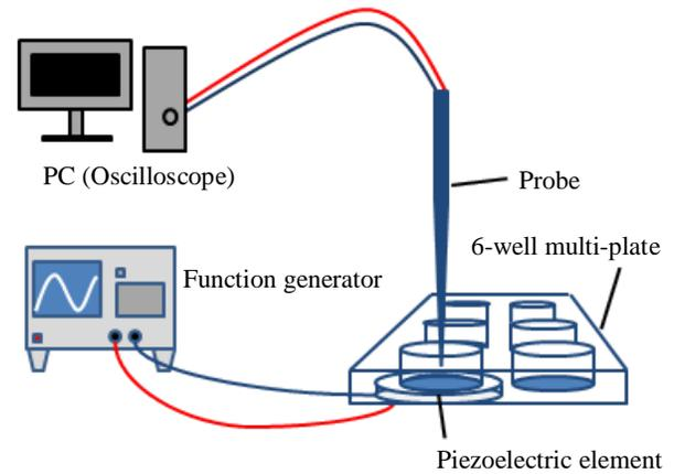
**Fig. 4:** Diagram of measurement of vibration in the medium.
