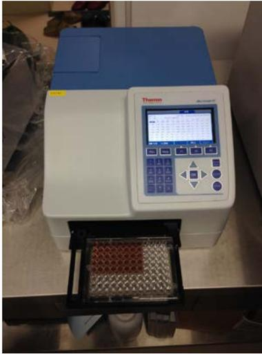
**Fig. 6:** Mounted samples in microplate photometer.
