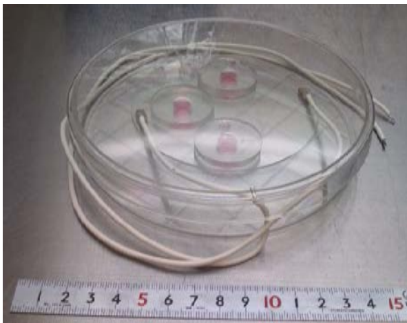
Fig. 3: Glass with ITO film in the dish of 100 mm diameter.
