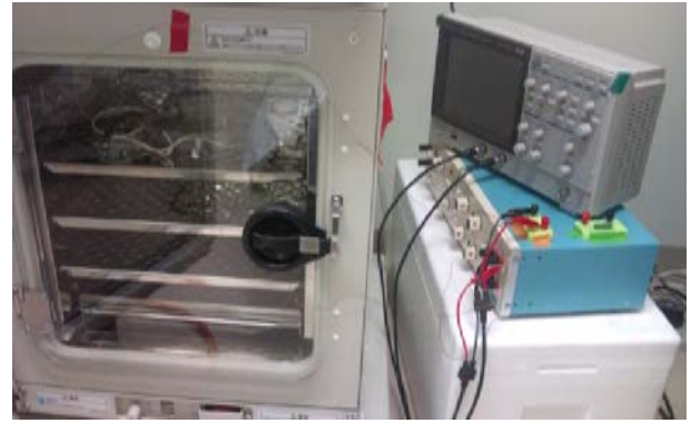
Fig. 4: Electric pulses introduced to scaffold of cells in incubator.
