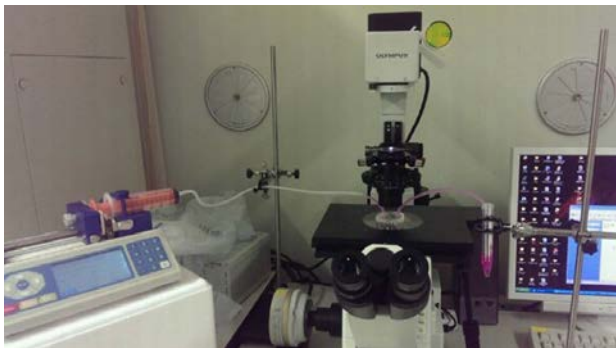
Fig. 2: Flow test system: flow chamber and microscope (middle), syringe pump (left).
