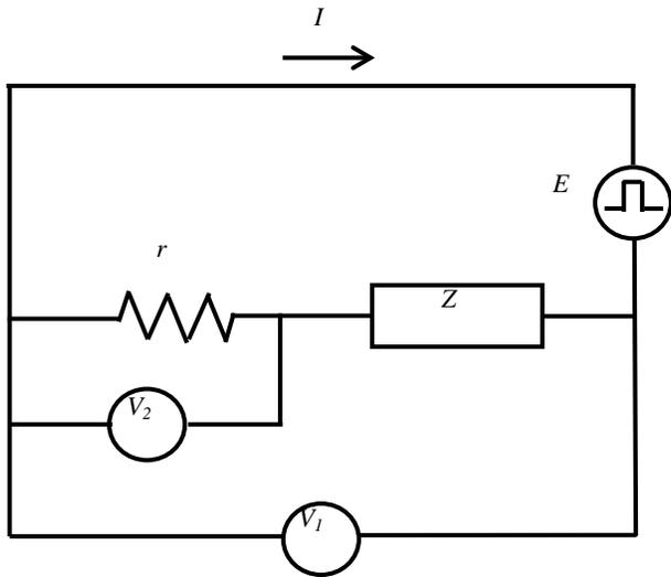
**Fig. 7:** Electric circuit:  $E$ , pulse generator;  $Z$ , medium;  $r$ , resistance;  $I$ , current;  $V$ , voltage.
