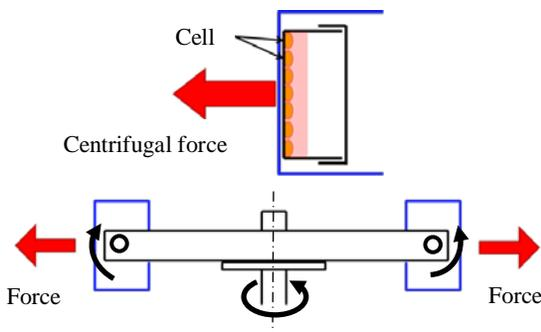
**Fig. 3:** Normal force on cell culture plane during centrifuge.
