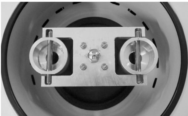
**Fig. 2:** Manufactured swing rotor in centrifugal machine.
