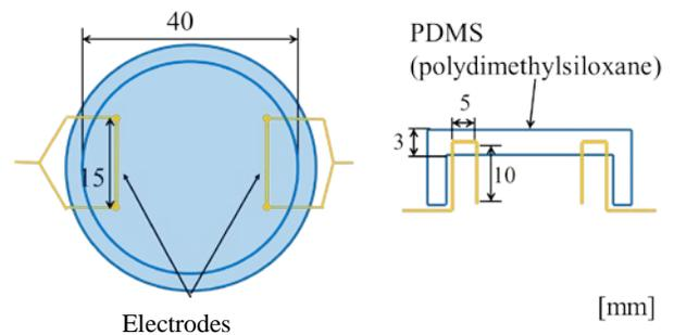
**Fig. 5:** Dimension (mm) of electrodes on cap.
