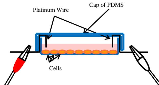
**Fig. 6:** Electrodes on cap of culture dish.
