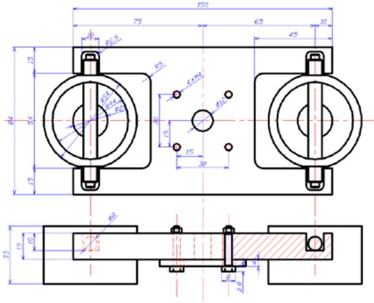
**Fig. 1:** Dimension (mm) of designed swing rotor.
