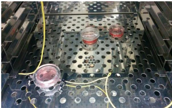
Fig. 6: Cell culture dish with electrodes in incubator.
