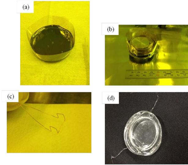
**Fig. 2:** Cap of PDMS with a couple of electrodes of Platinum wire. Top plate of cap (a), peripheral wall of cap (b), electrode of platinum wire (c), electrodes are fixed on cap (d).
