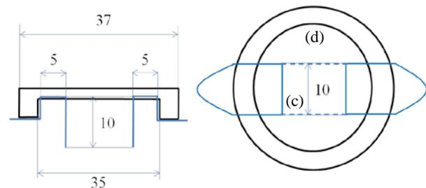
**Fig. 1:** Cap with a couple of electrodes (blue lines). Dimension in mm. (c) and (d) show the position for observation of cells (Figs. 11-15).
