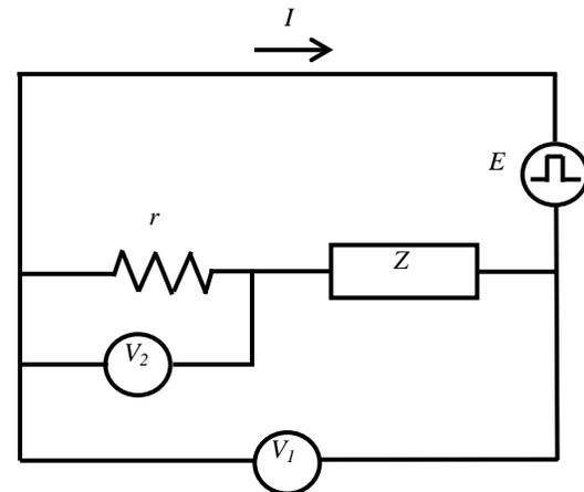
**Fig. 4:** Electric circuit:  $E$ , pulse generator;  $Z$ , medium;  $r$ , resistance;  $I$ , current;  $V$ , voltage.
