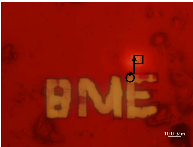
Fig. 5: Distance between the dissected point at the first trial (circle) and the targeted point at the second trial (square) of successive adjusting of dish. The square shows the target point for laser beam. The arrows show x and y coordinates, respectively.
