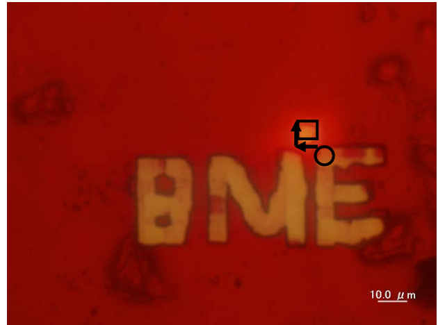
Fig. 6: Distance between the dissected point at the first trial (circle) and the targeted point at the third trial (square) of adjusting of dish. The square shows the target point for laser beam. The arrows show x and y coordinates, respectively.
