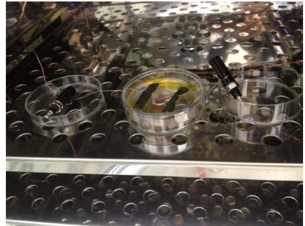
Fig. 3: Cell culture on micro coil spring with electric pulses.
