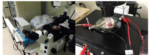
**Fig. 7:** Measurement of electric signal on stage of microscope (left) between electrodes (right).
