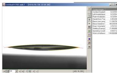
**Fig. 9a:** Contact angle on the film of ITO.
