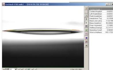
**Fig. 9b:** Contact angle on the base of the glass.
