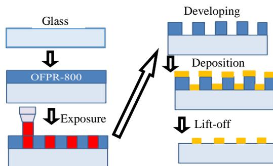
**Fig. 3:** Photolithography process for surface electrode.
