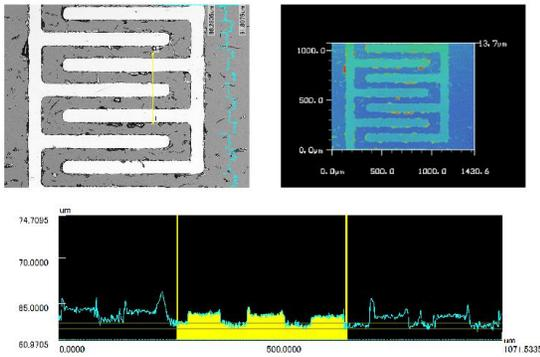
**Fig. 8:** Dimension of micro pattern measured with laser microscope.
