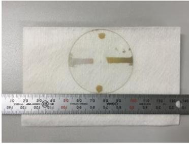
**Fig. 4b:** Surface electrodes on glass.
