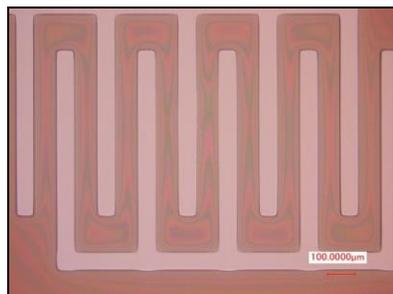
**Fig. 2:** Micro pattern of mask developed on the glass. Dimension from left to right is 1.3 mm.
