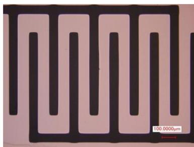
**Fig. 1a:** Micro pattern of mask for comb-shaped surface electrode. Dimension from left to right is 1.3 mm.
