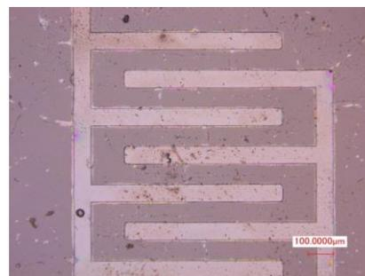
**Fig. 4a:** Comb-shaped surface electrode. Dimension from left to right is 1.3 mm.
