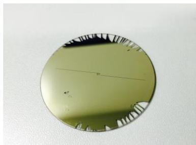
**Fig. 1b:** Photomask of titanium on the glass.
