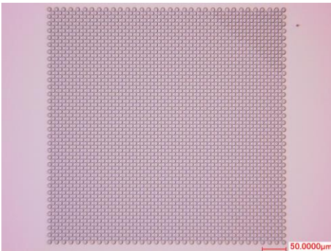
Fig. 5: Mold for micro-pillar array (without mask). Dimension from left to right is 0.7 mm.
