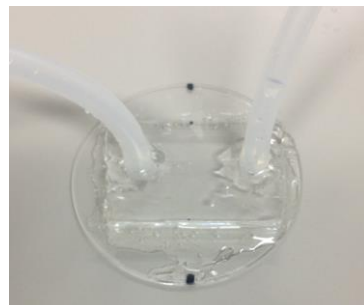
Fig. 7: Flow channel with micro slit.
