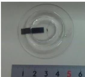
**Fig. 3b:** Manufactured electrodes of titanium film and spring.
