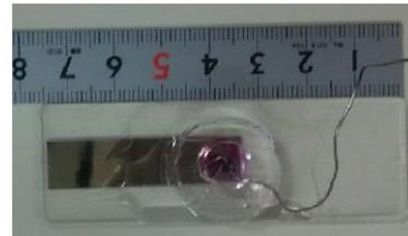
**Fig. 4b:** Manufactured electrodes of covered titanium film and wire.
