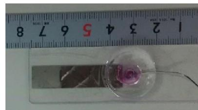
**Fig. 5b:** Manufactured electrodes of titanium film and wire.
