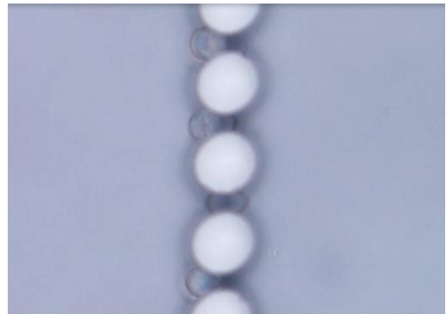
Fig. 8c: Deformed C2C12 goes through slit between micro cylindrical pillars ( w = 0.01 mm): diameter of cylinder is 0.025 mm: flow from left to right.
