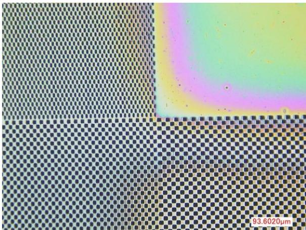
Fig. 3: Photomask after etching: dimension from left to right is 0.7 mm.
