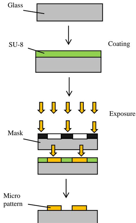
Fig. 4: Micro pattern on mold by photolithography.
