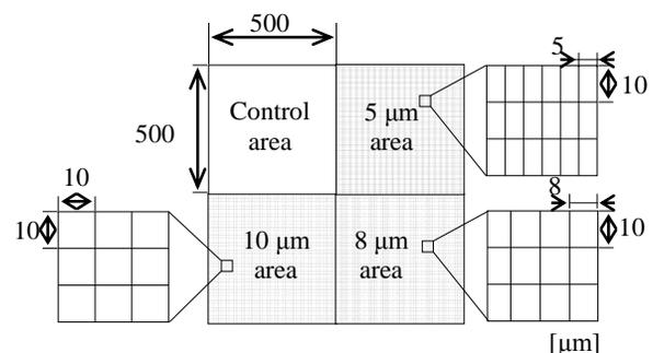
**Fig. 1:** Three kinds of checkered micro-pattern: aspect ratio of top rectangular surface of prism: 1 (lower left), 1.25 (lower right), 2 (upper right), and flat (upper left): mirrored pattern in Fig. 3, 5, 7, 8.
