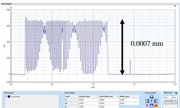
**Fig. 10:** Tracing (height [nm] vs. distance [mm]) measured by stylus on surface of mold.
