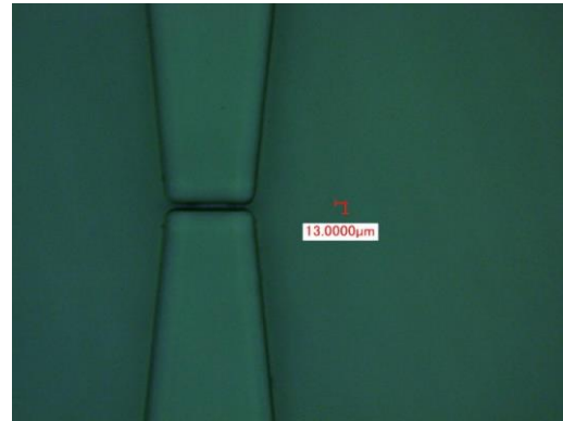
Fig. 6: Optical microscopic image of slit of SU8: dimension from left to right is 0.7 mm.
