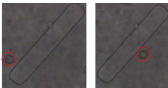
Fig. 10a: MC3T3-E1 (red circle) before groove (left), in groove (right); flow from left to right: optical microscope image.
