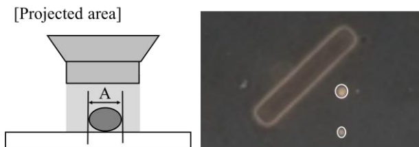
Fig. 8: Evaluation of dimension of cell (white circle) at optical microscope image (right).
