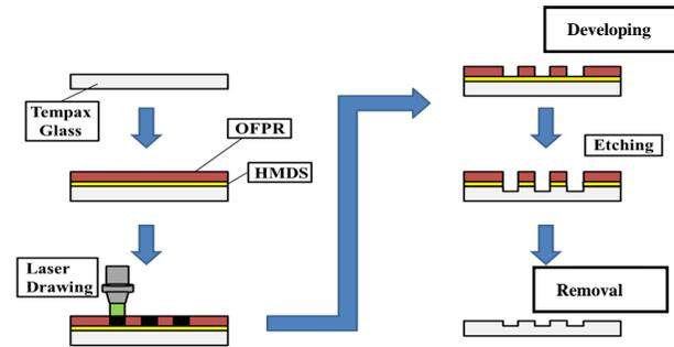
Fig. 2: Photolithography process for mold.
