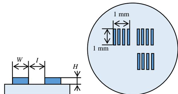
**Fig. 1:** Dimension of micro pattern (at cross section, left) in three areas on scaffold (right).
