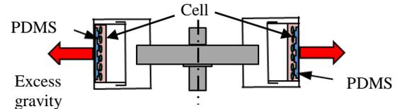
Fig. 4: Swing rotor in centrifugal machine.
