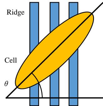
Fig. 7: Angle ( $\theta$ ) of major axis of cell related to longitudinal direction of micro ridge.
