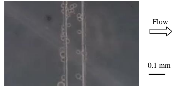
Fig. 4: Cells passing through slit: dimension from left to right is 0.8 mm; flow direction is from left to right.
