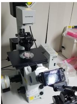
Fig. 2: Experimental system: channel, microscope, camera.
