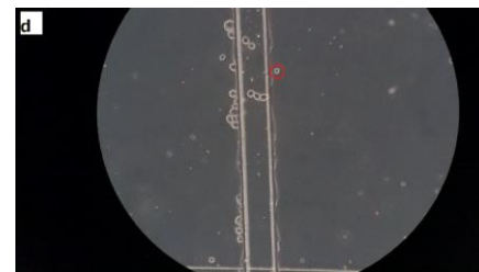
Fig. 5: C2C12 (in red circle) passing through slit: dimension from left to right is 2 mm: approaching to slit (a), passing through slit (c), departing from slit (d).
