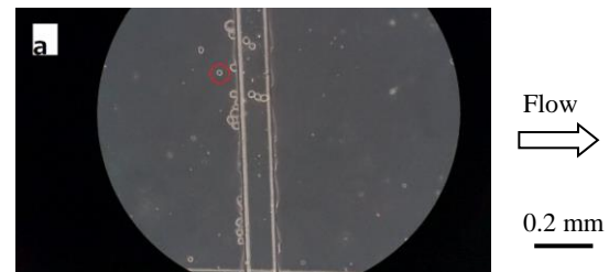
Fig. 4: Cells passing through slit: dimension from left to right is 0.8 mm; flow direction is from left to right.
