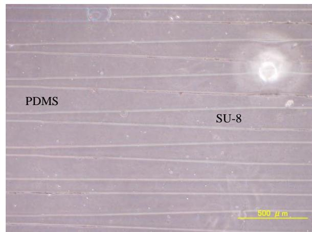
Fig. 3: Phase contrast microscopic image of hybrid taper-stripe pattern of SU-8 (0.05 mm – 0.15 mm) and PDMS (0.1 mm – 0.2 mm) for scaffold of cell culture. Dimension from left to right is 2.2 mm.
