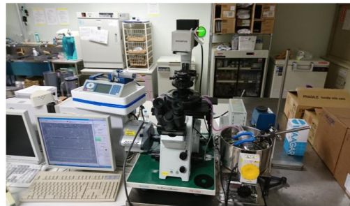
Fig. 4: Experimental system: syringe pump (left), flow channel on stage of microscope (middle), and reservoir in thermostatic bath (right).
