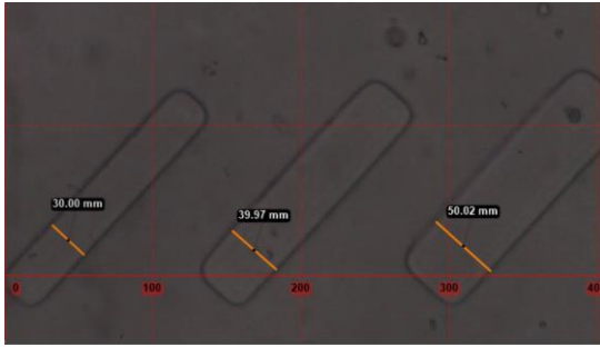
Fig. 4: Dimension of width of each groove. 0.05 mm
