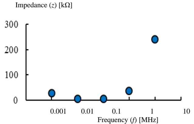
Fig. 7: Impedance  $z$  related to frequency  $f$ .
