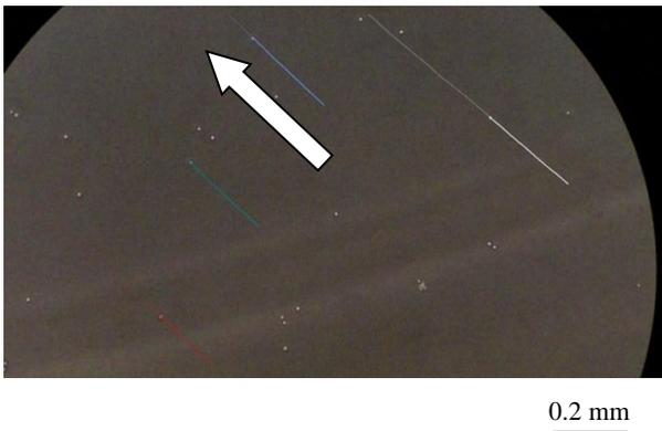
**Fig. 3:** Trappings of microspheres on surface of stationary plate in shear flow field: flow direction (arrow).
