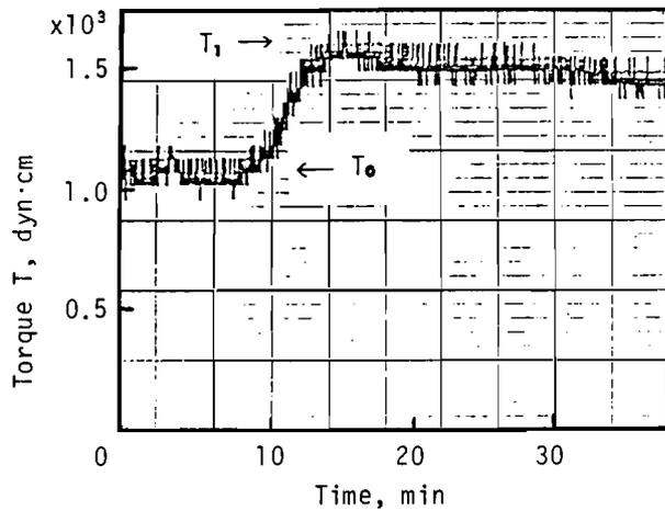
**FIG. 5.** Torque recording from the same test as that shown in Fig. 4 (polymethylmethacrylate cone and plate; angle between the cone and the plate  $\phi = 1.1^\circ$ ; shear rate =  $550 \text{ s}^{-1}$ ; preserved human blood).  $T_0$ , torque before formation of clot;  $T_1$ , torque after formation of clot.
