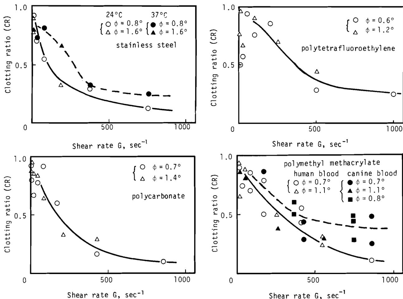
FIG. 7. Clotting ratio as a function of shear rate in blood between cone and plate made of stainless steel (top left), polytetrafluoroethylene (top right), polycarbonate (bottom left), and polymethylmethacrylate (bottom right).  $\phi$ , angle between the cone and the plate.
