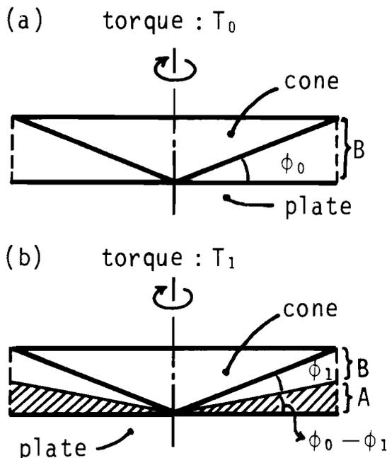
**FIG. 6.** Determination of clotting ratio in cone and plate viscometer tests before (a) and after (b) formation of clot. A, clot; B, blood;  $T_0$ , torque before formation of clot;  $T_1$ , torque after formation of clot.
