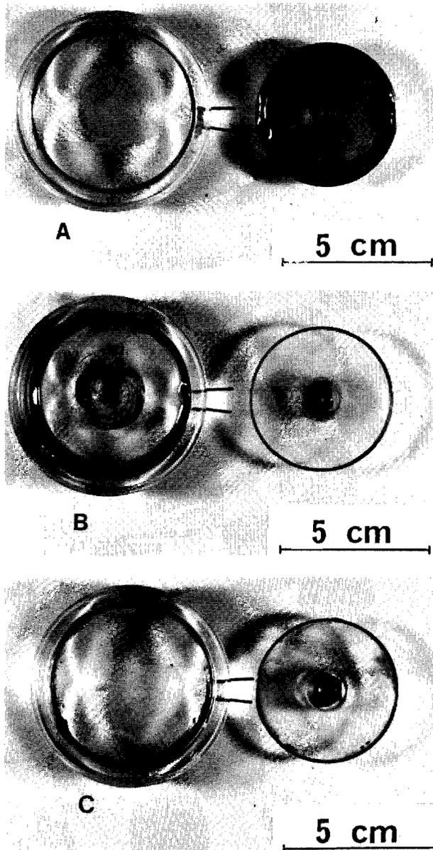
**FIG. 8.** Clot formed on the polymethylmethacrylate cone and plate (angle between the cone and the plate  $\phi = 0.7^\circ$ ; preserved human blood). The fluid part is removed after the test in the figure. **A:**  $G = 4.3 \text{ s}^{-1}$ ,  $CR = 0.90$ ; **B:**  $G = 43 \text{ s}^{-1}$ ,  $CR = 0.70$ ; **C:**  $G = 430 \text{ s}^{-1}$ ,  $CR = 0.45$ .  $G$ , shear rate;  $CR$ , clotting ratio.
