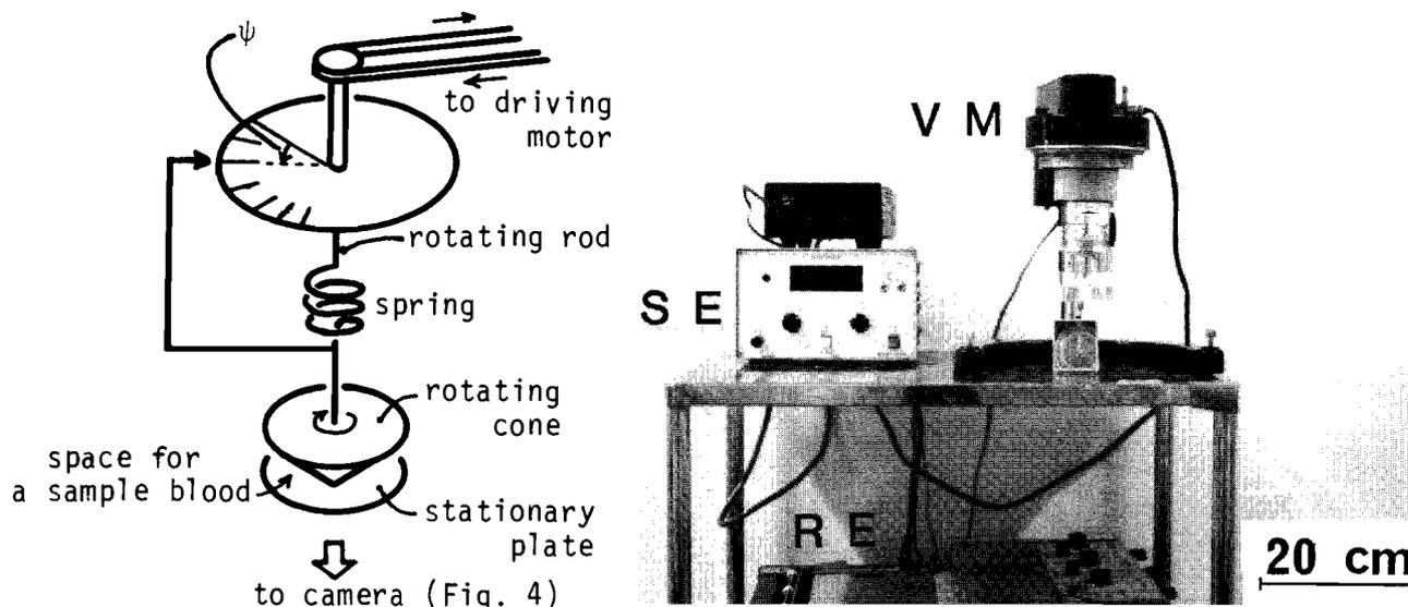
**FIG. 1.** Test equipment. **Left:** Schematic diagram of the cone and plate viscometer. **Right:** External appearance of the test equipment. The frictional torque is measured by the torsion angle ( $\psi$ ) in the spring attached to the rotating rod in the viscometer (VM) (right). The value of the angle  $\psi$  is picked up optically every rotation by the sensor (SE) and transmitted to the recorder (RE) (right).
