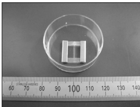
Fig. 1: Scaffold frame with polypropylene fiber.
