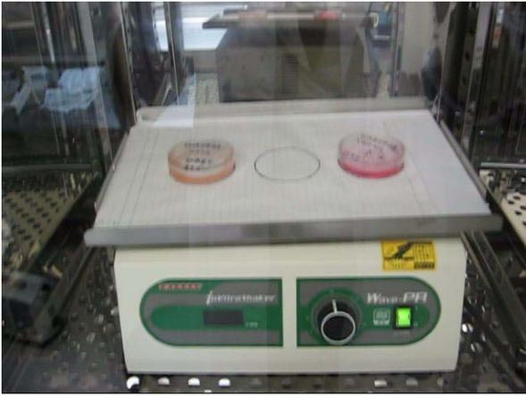
**Fig. 3:** Tilted rotating disk. Culture dish with (left) and without (right) silicone rubber sheet disk.
