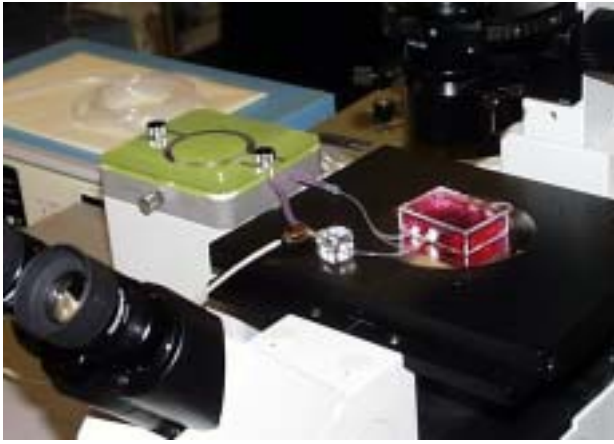
Fig. 10: The continuous flow was powered with a peristaltic roller pump.
