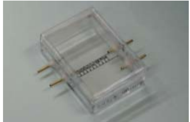
Fig. 8: Chamber made of the transparent styrene plate.
