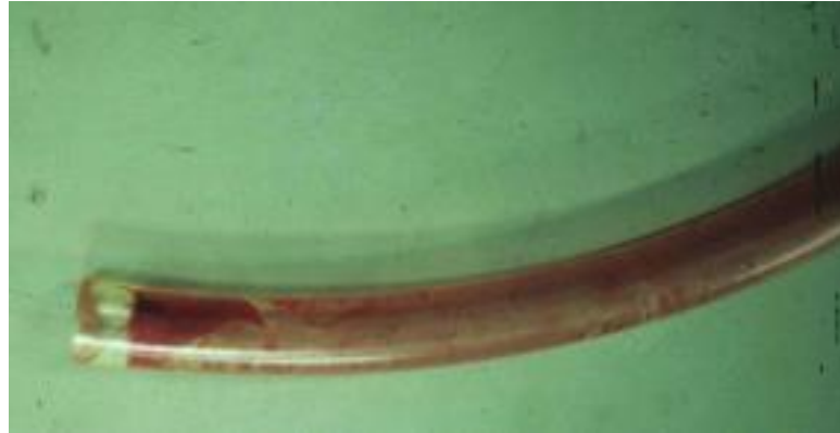
Fig. 6.25: Clot formation in tube (low flow)
