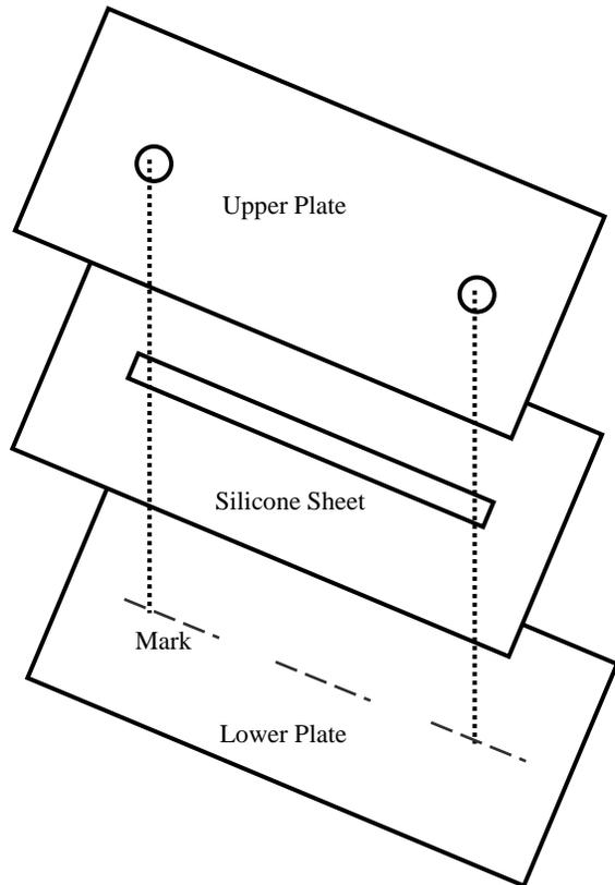
**Fig. 2:** Flow chamber of three plates; upper plates of glass, silicone sheet, lower plates of glass with mark.
