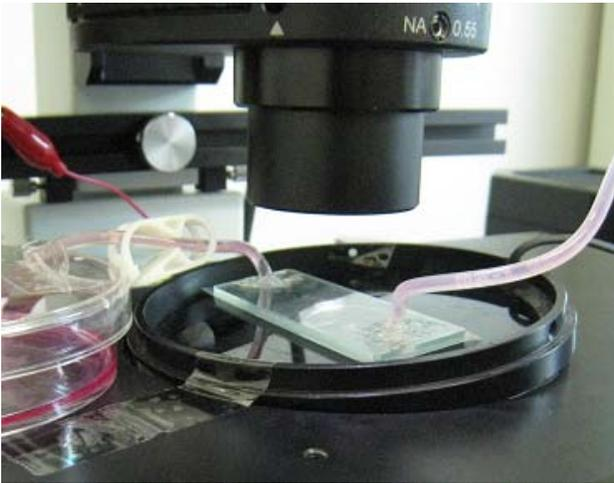
**Fig. 3:** Chamber placed on the tilted heating plate.
