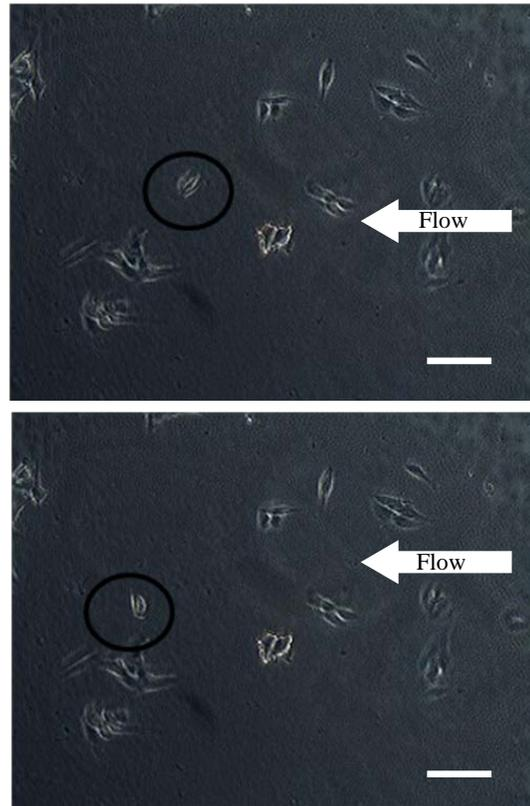
**Fig. 8:** L6 migrates downstream in 11 min under steady flow (from right to left) of 4 mL/hour. The bar shows 0.1 mm.
