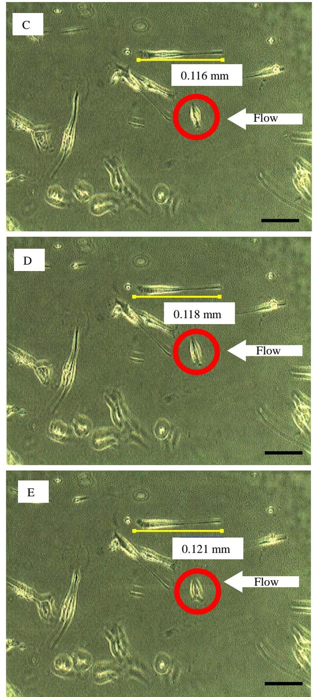
**Fig. 5:** C2C12 under steady flow (arrow: from right to left) of 4 mL/hour. Slope goes down from upper to lower. Cells were observed every 15 minutes: A, B, C, D, E.
