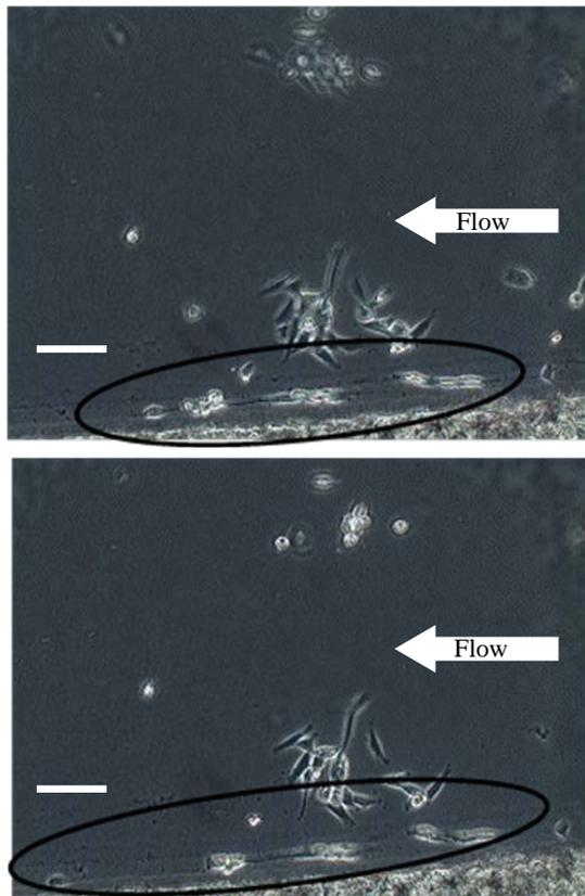
**Fig. 9:** L6 elongates downstream in 20 min under steady flow (from right to left) of 5 mL/hour. The bar shows 0.1 mm.
