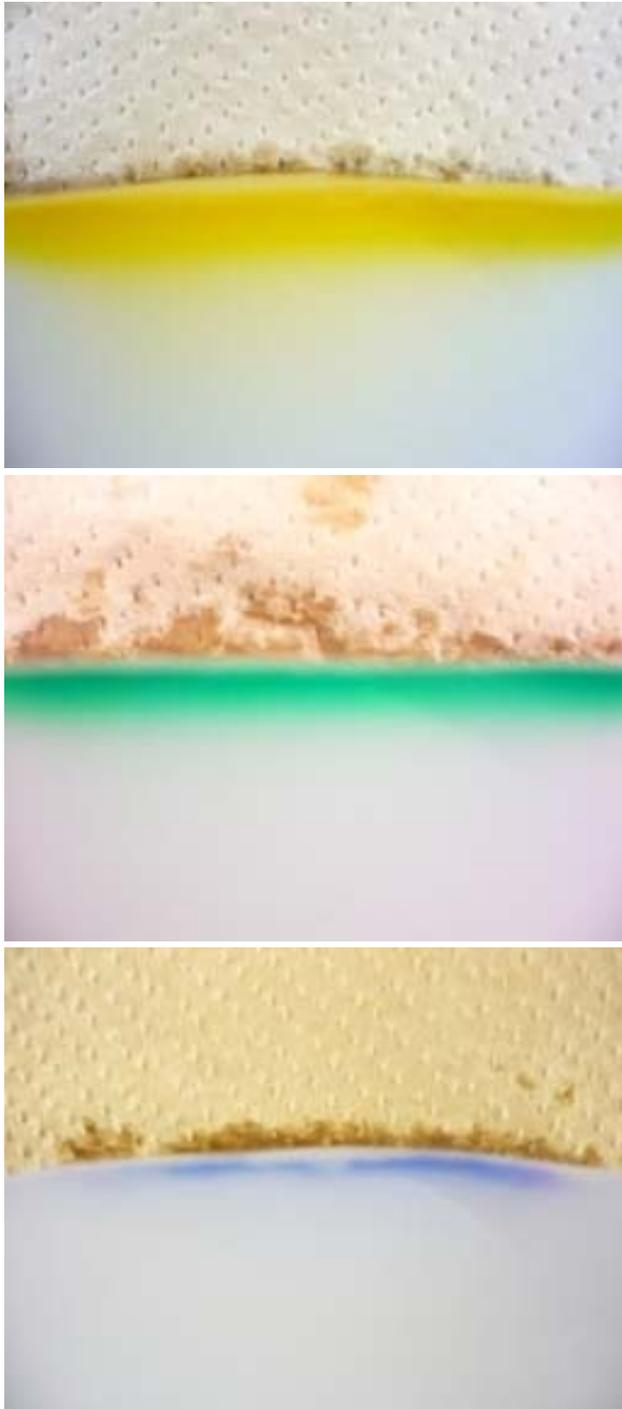
**Fig. 3:** Penetration from top to bottom: upper, phenol red; middle, brilliant blue FCF; lower, trypan blue. (Pulse of 5000 Hz, 60 min)
