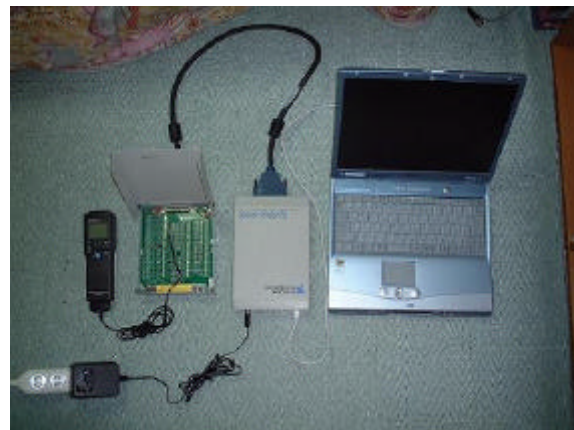
Fig. 5: Radiation thermometer sensor (left), multifunction data acquisition (middle), computer (right).
