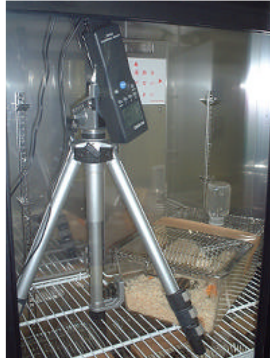
Fig. 4: Telemetric measurement of surface temperature of the squirrel with radiation thermometer (upper left): cage (right).
