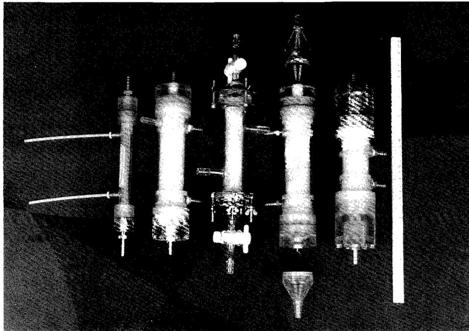
FIG. 2. Pneumatic pulse pump membrane oxygenator in tube type: models 1, 2, 3, 4, 5 (from left to right). In models 1-3, one-way valves are removed. In model 5, ball valves are built-in.
