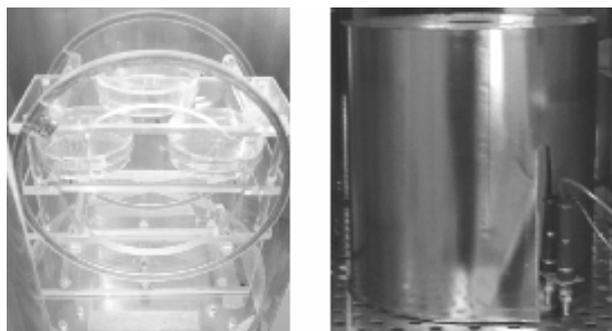
**Fig. 4:** (a) Helmholtz coil (dishes parallel to the magnetic field), (b) Magnetic shield.
