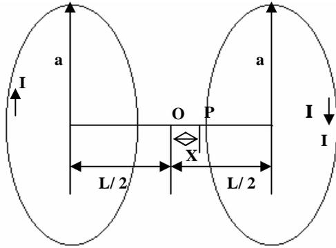
Fig. 7: Two circular coils.
