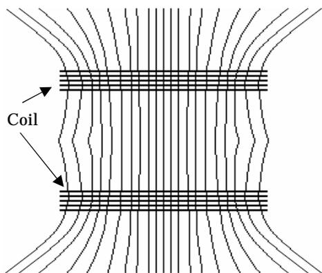
**Fig. 2:** Magnetic field between two coils.
