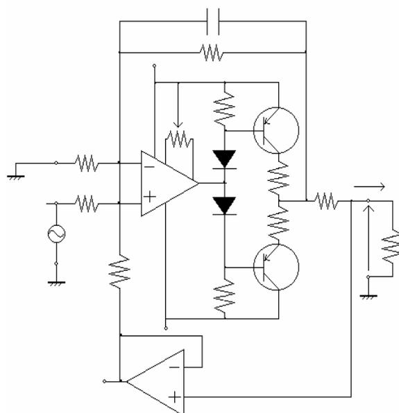
**Fig. 5:** Circuit diagram of converter from voltage to electric current.
