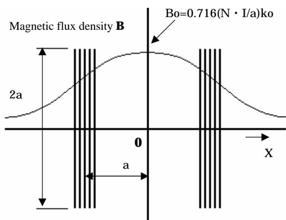
**Fig. 3:** Magnetic flux of Helmholtz coil.
