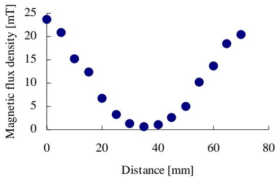
**Fig. 3:** Magnetic flux density in relation to distance from the right end of the left coil.
