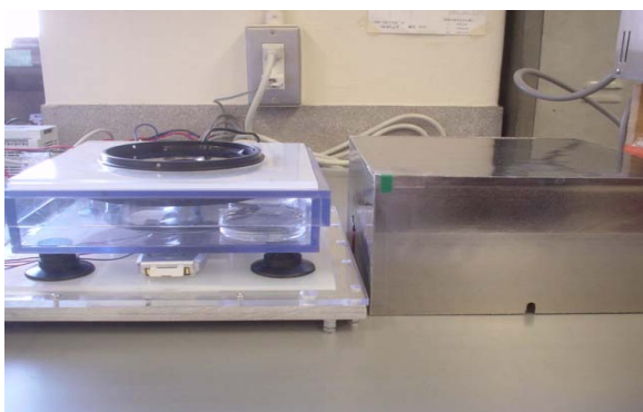
Fig. 3: Chamber of incubation (left), Electromagnetic shield (right).
