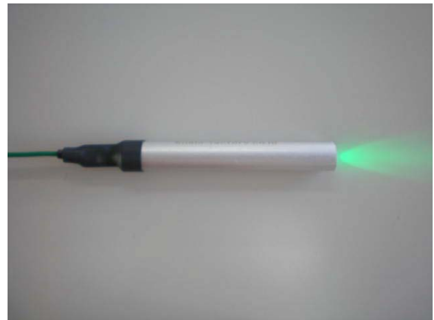
Fig. 1: Green light emitting diode.
