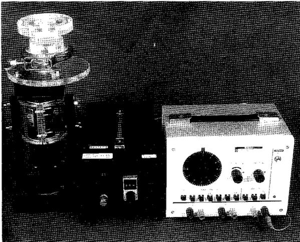
FIG. 1. Test system. Left, concavo-convex testing machine; rotating-speed controller; right, function generator.
