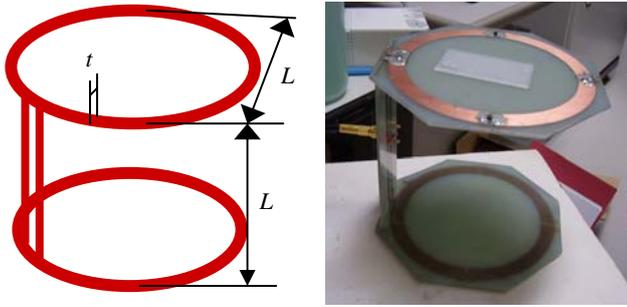
**Fig. 7:** Helmholtz coil (wireless coil)
