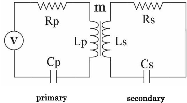
**Fig. 2:** Equivalent circuit of dual coils.
