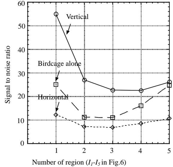
**Fig. 12:** Signal to noise ratio in each region ( $I_1$ - $I_5$  in Fig. 11)
