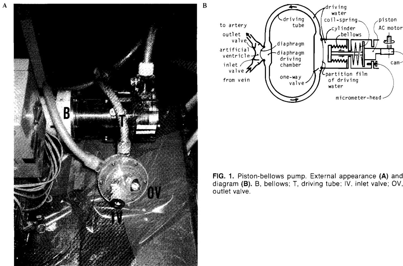
FIG. 1. Piston-bellows pump. External appearance (A) and diagram (B). B, bellows; T, driving tube; IV, inlet valve; OV, outlet valve.
