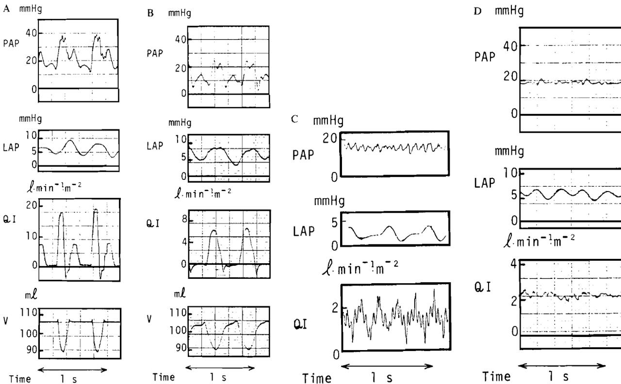
FIG. 7. Some examples of simultaneous traces of pressure and flow during total right ventricular bypass with three types of pumps. A and B, piston-bellows type (A, ER = 7.5 mm; B, ER = 2.5 mm); C, screw type; D, centrifugal type.
