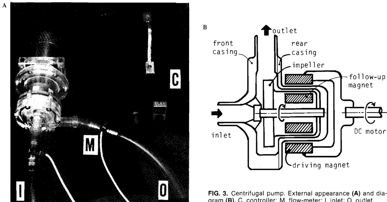
FIG. 3. Centrifugal pump. External appearance (A) and diagram (B). C, controller; M, flow-meter; I, inlet; O, outlet.
