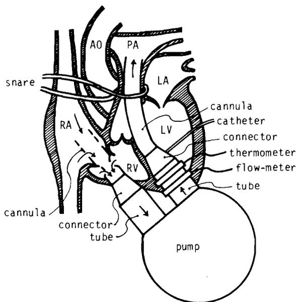
FIG. 4. Cannulation method of the total right ventricular bypass. RA, right atrium; RV, right ventricle; PA, pulmonary artery; LA, left atrium; LV, left ventricle; AO, aorta.
