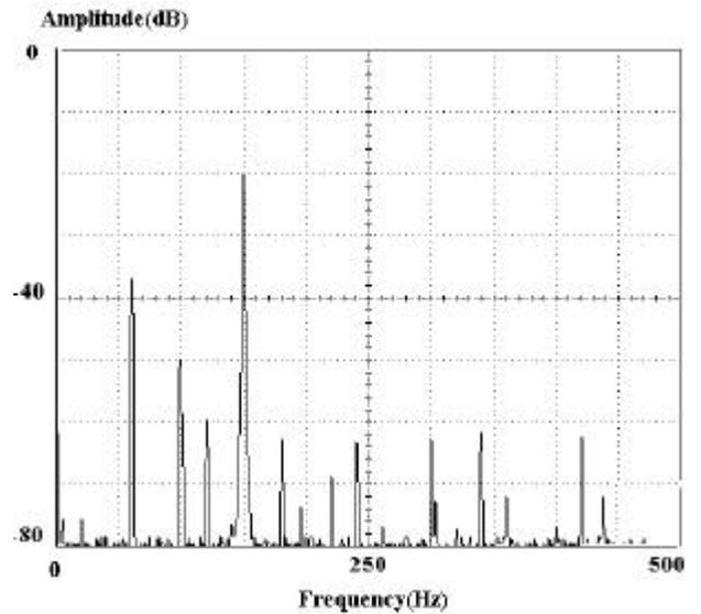
**Fig. 11(c):** Power spectra of the output voltage with the medium. The electrode was vibrated at 100 Hz. The input voltage was oscillated at 150 Hz. The spectra at 60 Hz, 100 Hz and 150 Hz correspond to noise from the electric source,  $A V_{dx}$  and input signal, respectively.
