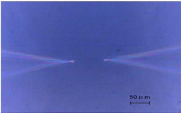
**Fig. 3:** Micro-electrode. Schematic diagram (A), and the tips of micro-electrodes under microscope (B).
