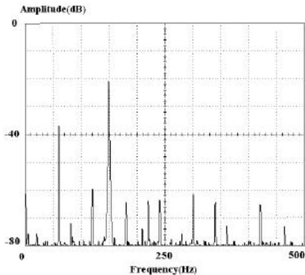
**Fig. 11(a):** Power spectra of the output voltage with the medium. The electrode was not vibrated. The input voltage was oscillated at 150 Hz. The spectra at 60 Hz and 150 Hz correspond to noise from the electric source and input signal, respectively.
