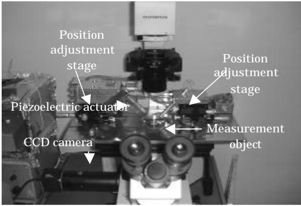
**Fig. 5:** Microscope and stage.
