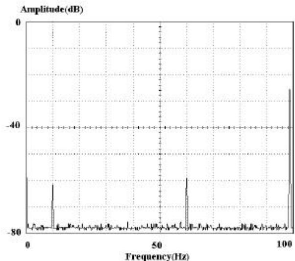
Fig. 10(a): Power spectra of the output voltage with saline solution. The electrode was vibrated at 10 Hz. The input voltage was oscillated at 100 Hz. The spectra at 10 Hz, 60 Hz and 100 Hz correspond to  $A V dx$ , noise from the electric source and input signal, respectively.
