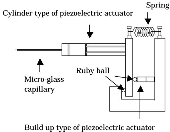
Fig. 8(b): Constitution diagram of scanning probe.
