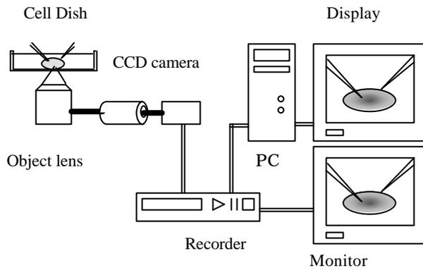
**Fig. 6:** The diagram of capturing the image of the tips of electrodes.
