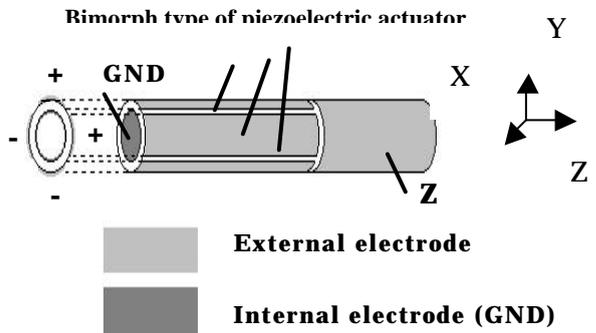
**Fig. 7(b):** Cylinder type of piezoelectric actuator. This actuator consists of four external electrodes, one internal electrode and build up type of electrode. Movement in X (or in Y) direction is controlled with voltage between opposite external electrodes.
