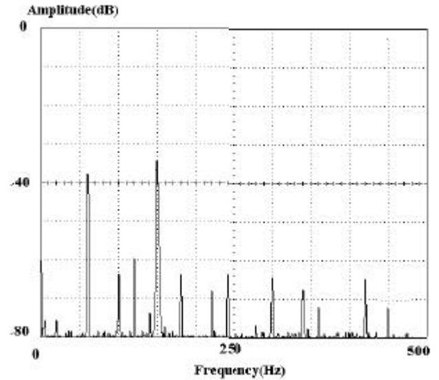
**Fig. 11(b):** Power spectra of the output voltage with endothelial cell. The electrode was vibrated at 100 Hz. The input voltage was oscillated at 150 Hz. The spectra at 60 Hz, 100 Hz and 150 Hz correspond to noise from the electric source,  $A V_{dx}$  and input signal, respectively.
