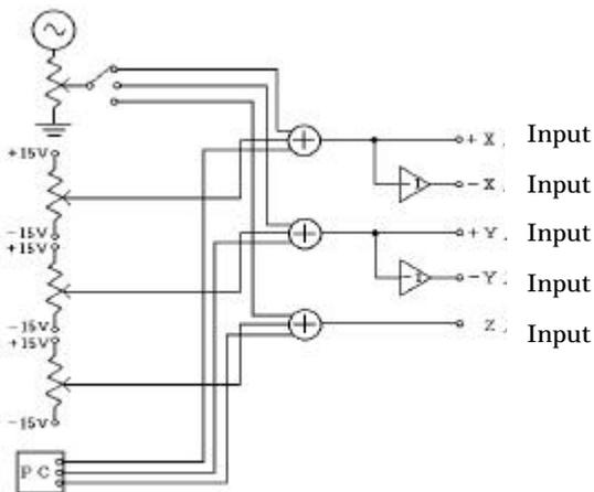
Fig. 9: The circuit of the probe controller.
