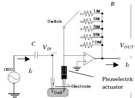
**Fig. 4:** The electric circuit of the measurement system.  $V_{in}$  is input signal applied to the biological tissue and  $V_{out}$  is amplified output signal.  $R$  is varied with the switch.
