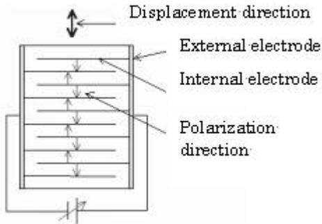
Fig. 8(a): Build up type of piezoelectric actuator.
