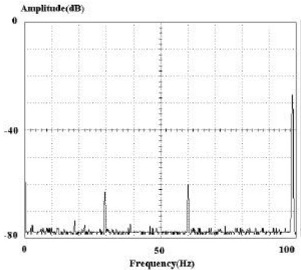
**Fig. 10(b):** Power spectra of the output voltage with saline solution. The electrode was vibrated at 30 Hz. The input voltage was oscillated at 100 Hz. The spectra at 30 Hz, 60 Hz and 100 Hz correspond to  $A V_{dx}$ , noise from the electric source and input signal, respectively.
